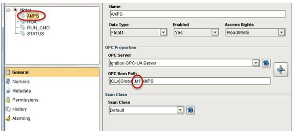
Because we are creating a UDT, we don't want to point to one specific set of Tags. We want each instance of the UDT to reference a different set of Tags. To do that, we need to add a parameter to the UDT. Parameters are custom properties on data types. You can use the parameters inside the type or instance definition to create parameterized data templates.
