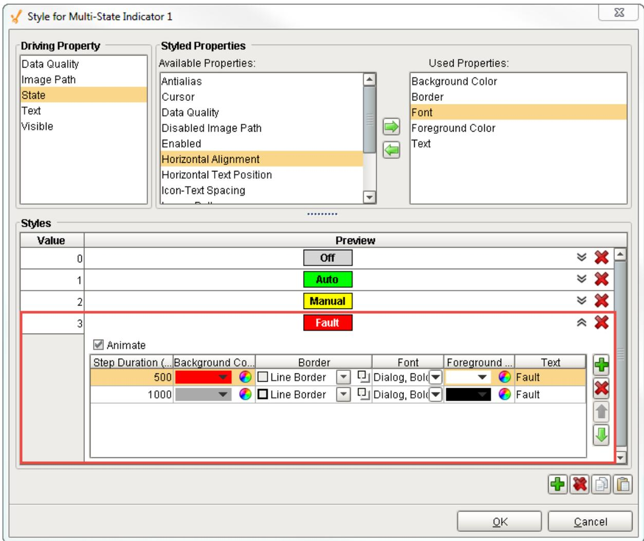
6. Change the **State** to '3' to see the component blink **'Faulted'** and switch between the background and foreground colors you setup.
